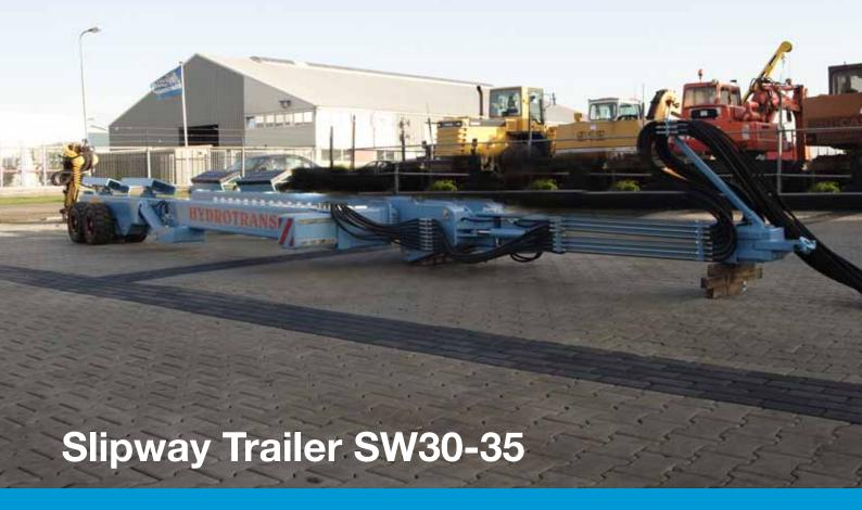
The Hydrotrans hydraulic boat trailer is designed to launch and recover boats on a slipway, transport the boats over land and park them in a storage or work area.
