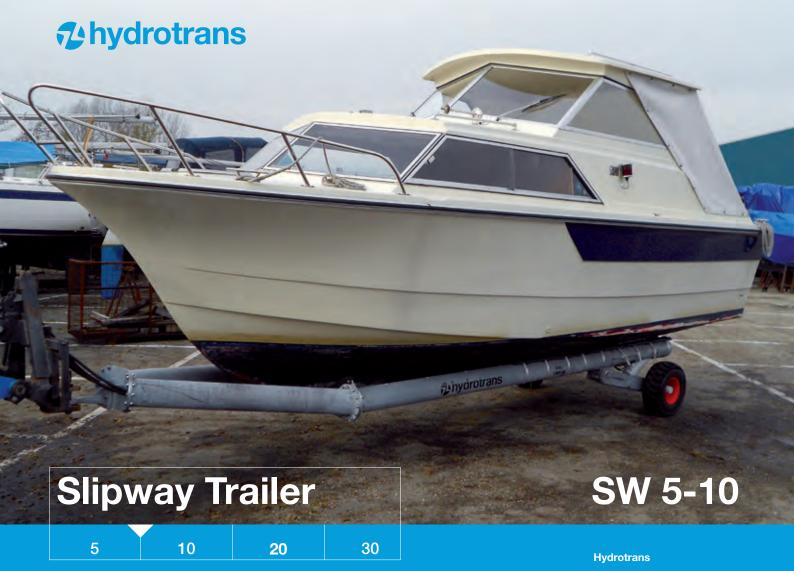
The Hydrotrans hydraulic boat trailer is designed to launch and recover boats on a slipway, transport the boats over land and park them in a storage or work area.
